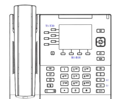
The Mitel 6867 consists of handset, screen, navigation/select key, numpad, option keys, line keys (L-keys) and softkeys (T-keys and B-keys).
