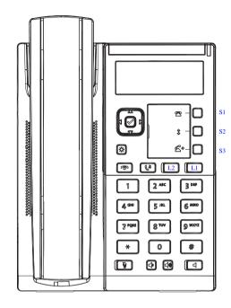
The Mitel 6863 consists of handset, screen, navigation/select key, numpad, option keys, line keys (L-keys) and softkeys (S-keys).
